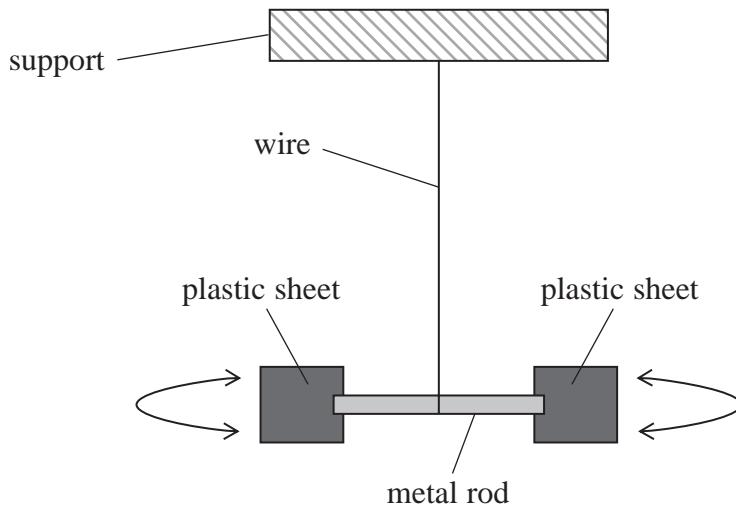
When the metal rod is rotated through an angle and released, the rod performs angular oscillations about a vertical axis through the wire. The plastic sheets dampen the oscillations as they move through the air.
